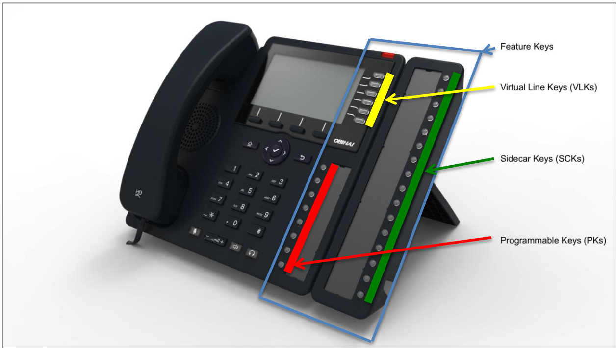
Figure 13: Diagram of OBi1062 with OBi1000e sidecar showing the location and types of feature keys
