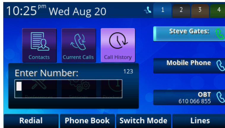
Figure 19: GUI screen showing a Dial Dialog during off-hook dialing with the handset. Note the handset icon in the status bar.
