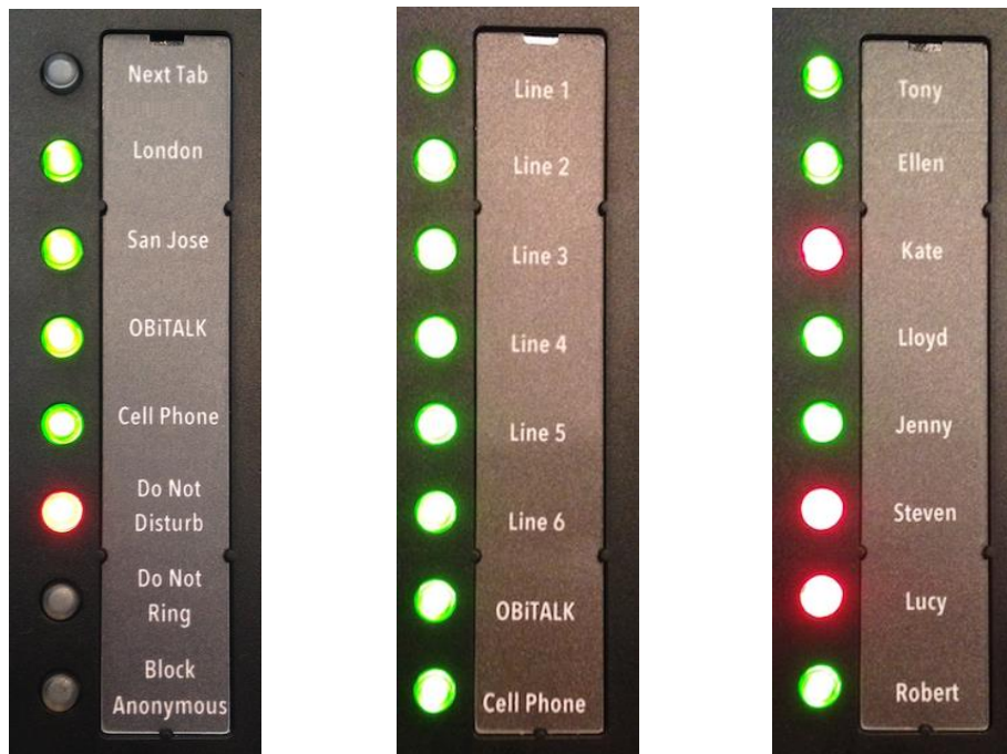
Figure 17: Three examples of possible layouts for the programmable keys (PKs).
